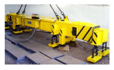
For customers that need to lift various sheet dimensions, the Magswitch Telescoping Lift System offers adjustability based on the length of the plate being handled.
