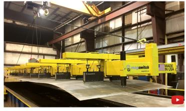
Designed to lift your maximum plate size, the Magswitch Fixed Lift System can be configured with any number of cross members to fit your lifting needs. With zone control, independent activation of cross members allows for picking of varying plate sizes.
