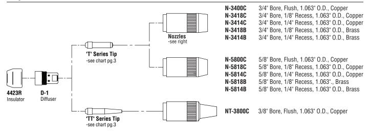
Diffusers, nozzles and contact tips are available in packages of 10 and insulators are available in packages of 5
