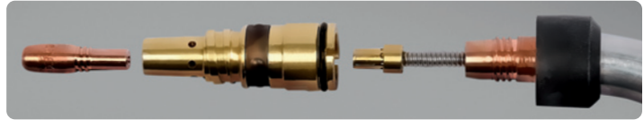
Front-loading AccuLock liner locks at front and back of gun to align with contact tip and power pin for a flawless wire-feed path (AccuLock S consumables shown)
