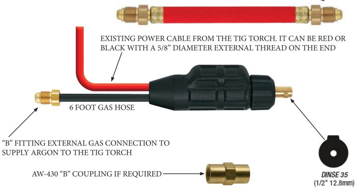
THE SL5-35 IS AN EXTERNAL GAS AND POWER CABLE CONNECTOR. YOU NEED TO KNOW HOW THE GAS IS GOING TO GET TO THE TIG TORCH.
