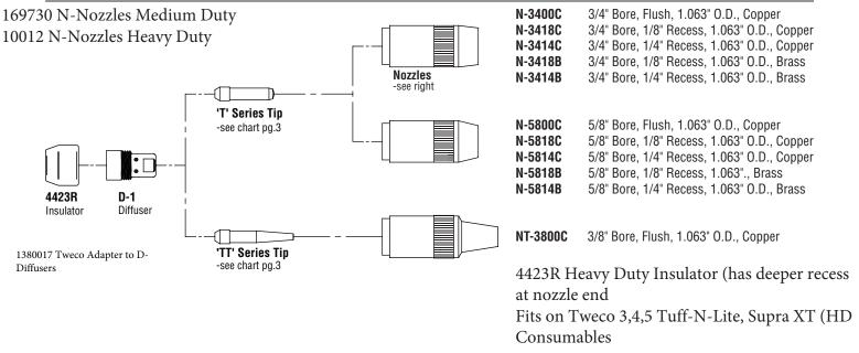
Diffusers, nozzles and contact tips are available in packages of 10 and insulators are available in packages of 5
