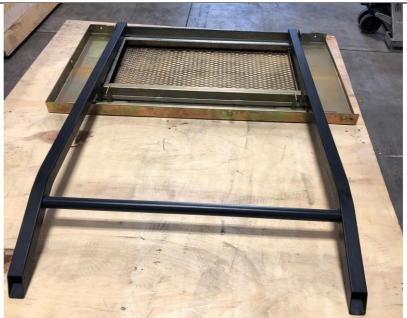
Take the longer of the two table legs and place on top of the table work surface to align with the wider set of pivot clips on the table work surface. Table leg ends should be pointing down.
