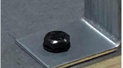
Place the slag tray handle to align with the predrilled holes in the slag tray. Put a flat washer 6 on the M6 x 12MM hex head bolt and push through the holes in the handle and the tray.
