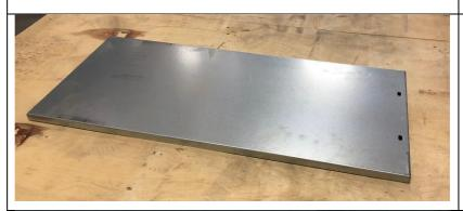
Place the removable slag tray on a sturdy surface, with the flat side (bottom) up.
