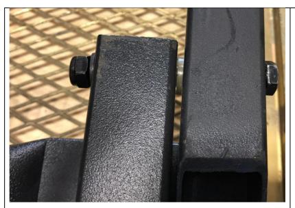
Install the hardware through the mounting hole in the short table leg and the mounting hole through short table leg extension. Hand-tighten only, tighten only after table assembly is complete.
