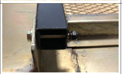
Install the hardware through the hole in the pivot clip and the hole through the leg.
