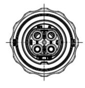
Wire Range: #4 - #8 AWG Cord Range: .50" - 1.45" Threaded Cable Entry: 1 1/2" NPT
