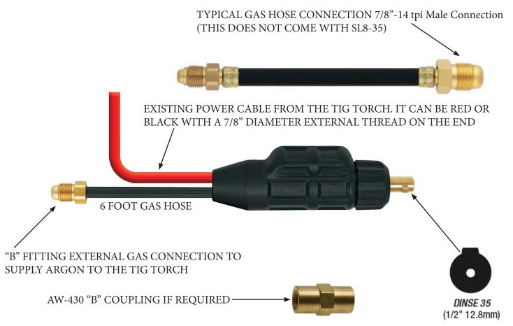
THE SL8-35 IS AN EXTERNAL GAS AND POWER CABLE CONNECTOR. **YOU NEED TO KNOW HOW THE GAS IS GOING TO GET TO THE TIG TORCH.**
