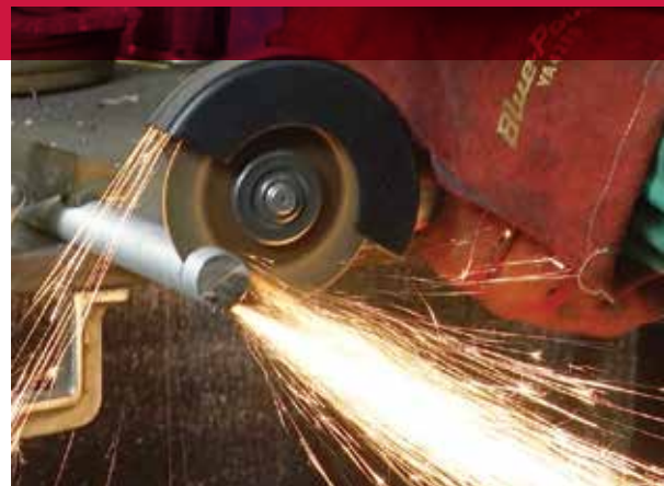
Cutting a piece of bar stock with an UltraCut wheel.
